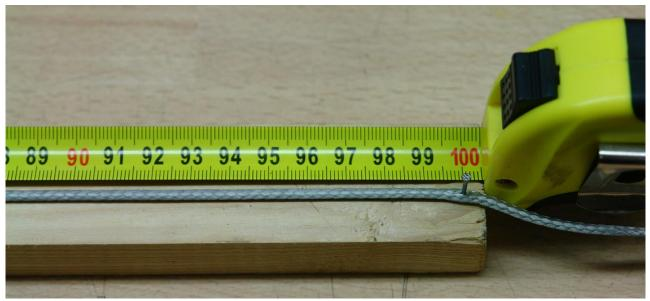
Use a felt pen with a thin tip to mark the line at the calculated positions. In case you want to make several equally DD Vari Loops Then you can mark the wooden slat as well and use it in future as stencil
