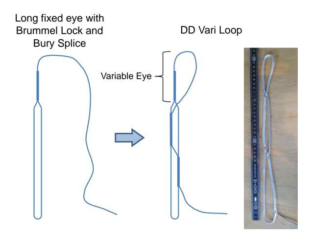
Basically a long fixed eye is modified with two extra burysplices, transforming it into a DD Vari Loop
